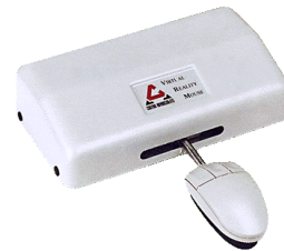
Figure 4 – Virtual Reality Mouse provides force feedback using a gravity interface. The mouse resists crossing boundaries such as window borders, and gently draws the user toward possible targets like icons. This pointing solution exaggerate the pointer's interaction with the interface.
