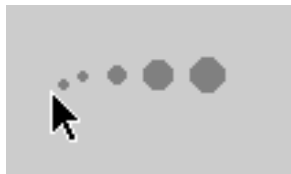
Figure 6 – Cursor Comet. A comet tail falls off behind the mouse pointer. The length of the tail is a function of speed. When moving rapidly across the screen, the visual effect of the tail exaggerates the pointer's motion. This makes the pointer's path easier for the user to follow.
