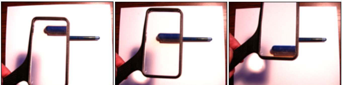
Figure 2. Motion effect of magnification: as the magnifier moves upwards, the magnified image moves down.
