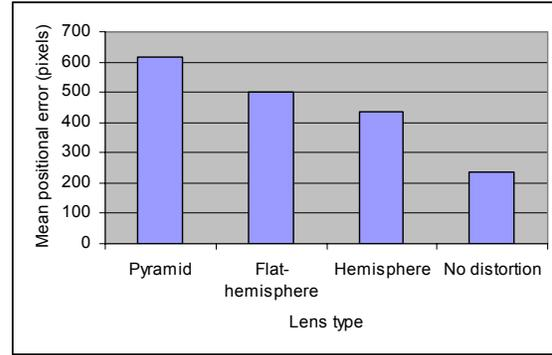
Figure 7. Mean positional error per figure for all lens types at all distortion levels. The no-distortion baseline is shown for comparison but was not included in the analysis.
