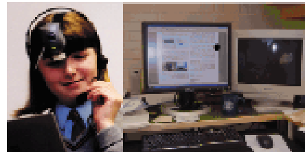
Figure 8. A head mounted camera (left) and one of its possible captures (right).
