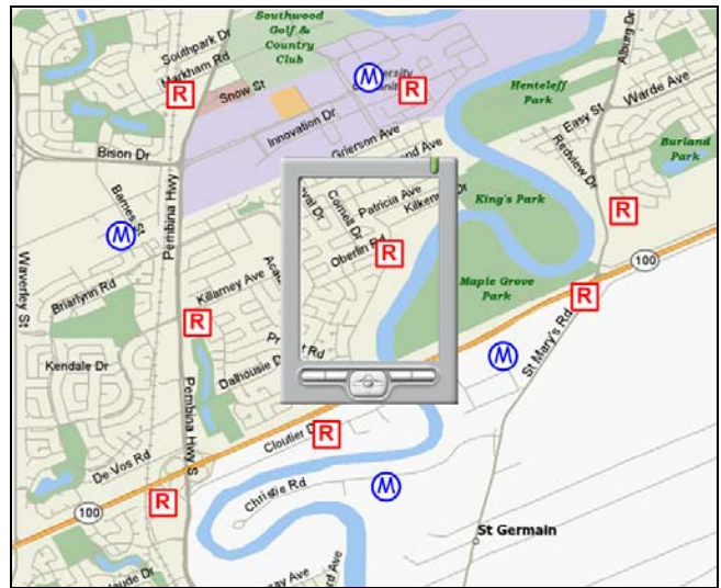
Figure 1. Large visual workspace with several candidate targets (R=Restaurants; M=Metro Stations), with PDA viewport superimposed.
