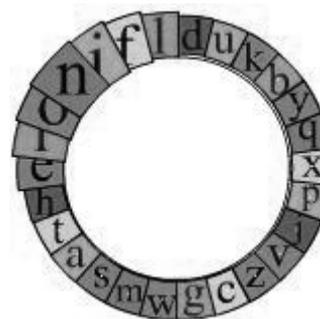
**Figure 2. Expanding CIRRIN with 60% expanding targets. Notice that the largest button, and all partially expanded buttons overlap nearby smaller buttons, showing the occlusion model.**
