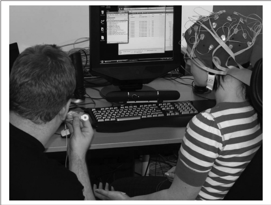
Figure 4. The electrodes are applied to a participant and EEG electrodes are placed on scalp locations with a cap
