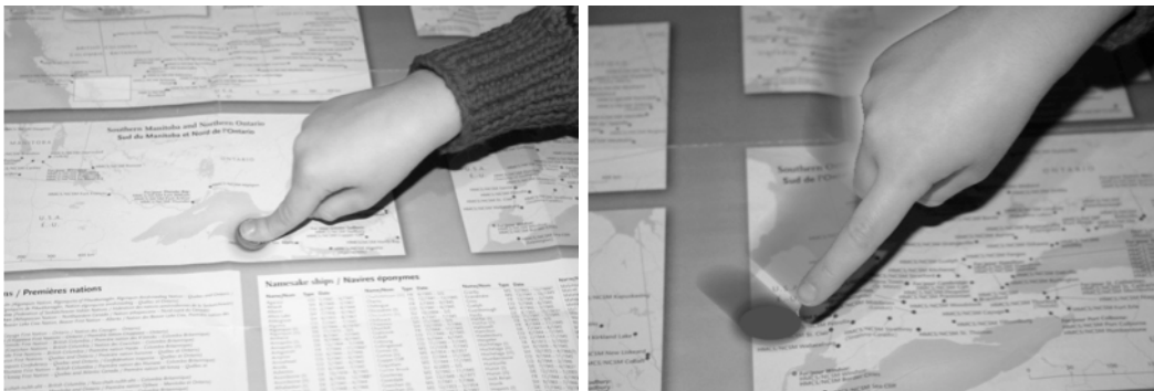
Figure 4. A mock-up of elements of a hybrid visualization. Left, a coloured ripple effect enhances the contact point and provides pressure information. Right, temporal traces emphasize a stroke atom and a ray-cast shadow at the pointing target provides height information.
