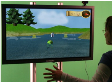
Figure 3. The Frog Prince (part of the Wuppd! suite) is a single player game which requires wide circular arm movements, similar to breast-stroke swimming. Synchronous movement of both arms controls forward motion, movement of a single arm controls turns.
