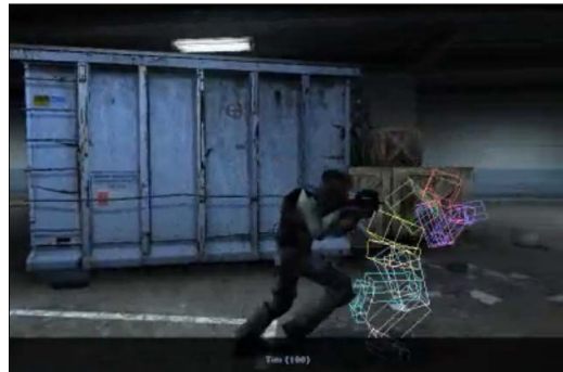
Figure 1. Frame from Counter-Strike: Source . Wireframe ‘hitboxes’ show server location of avatar; local representation is lagged.
