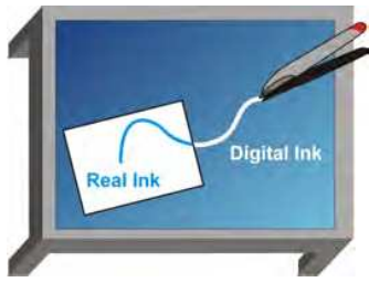
Figure 2. A hybrid pen writes with real ink on the palette surface and acts as digital input on the augmented tabletop (which is covered with an ink-repellent layer)
